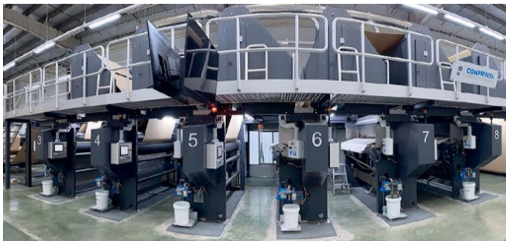
The showpiece: the latest CONPRINTA IMD2200, a 5-color flexographic web printing system plus varnishing system
